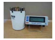
We can also test total normal reflectance on the AZ Technology Temp 2000A. A calculated normal emittance value can be provided by testing on the AZ Technology Temp 2000A Reflectometer in the Relative Mode. This meets meets ASTM-E408 Method B.
