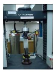
All tapes sold by Sheldahl are tested for bond strength. This test is done by applying the tape to a clean stainless steel substrate using a prescribed pressure and then measuring the force required to remove the tape using an Instron instrument. Our test methodology is in accordance with ASTM D-1000 and ASTM D-3330. We can also test adhesion to aluminum plates if desired.
