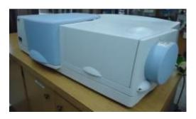
Sheldahl measures solar absorptance using a Perkin-Elmer Labsphere 950 UV-VIS-NIR spectrophotometer.
